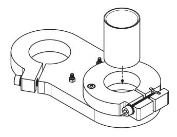
Assemble the magnets on the last PMMA part as shown with the two M3x10 screws.
