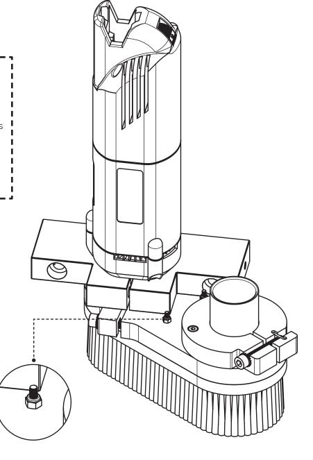
USE THE DUST SHOE ONLY IF THE MAGNETS STICK CORRECTLY TO THE WASHERS (if it's not the case, refer to the note above)
