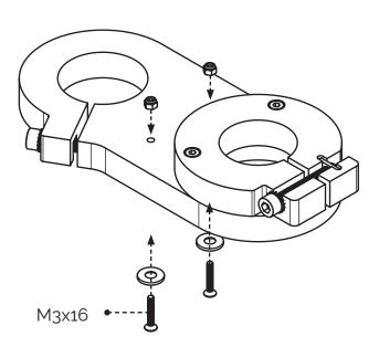
Place the plastic adaptator into the clamping ring and tighten it.
