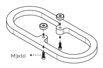
6 Insert the brush\* part in the slot as shown.
