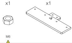
Simply place the M6 nut inside the triangular pocket
